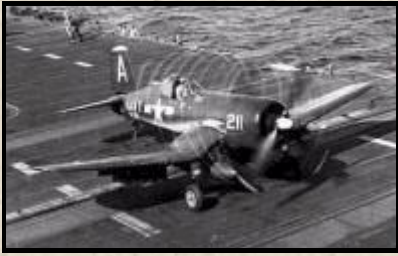
This picture of a WW2 Corsair clearly shows that the prop imparts a swirl to the airflow, causing it to hit the fin at an angle. This produces a yawing force, typically causing the nose to want to swing to the left.
