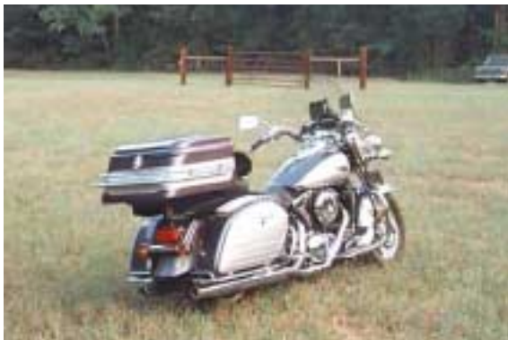
Tour Pack Trunk mounted on a 2001 Nomad, using the Scootworks trunk mounting kit.
