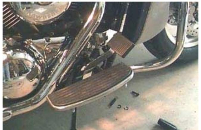
**6.** The photo above (left) shows the lever installed with the arm parallel to the floor. This is the position preferred by many riders. Shorter riders who want the floorboard space, but need the pad tilted towards the riding position for easier access, may engage the lever's splines at a slightly different location to achieve this. Observe, as in the photo on the right...
