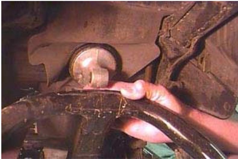
**9.** The upper end of the shock is secured via large allen bolt and 17mm hex nut, in the frame down tube, just behind the engine. Some bikes require a 6mm allen wrench, some require a 8mm allen wrench. Remove the 17mm nut, then screw the allen bolt from the down tube. The shock should be easily removed by pulling rearward gentle rocking left and right.
