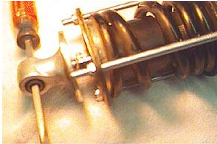
Install the new Scootworks Shock Head (adjustable lowering kit) on the shock. Screw the adjustable lowering kit **all the way down** and onto the shock rod. Tighten the locking nut, and remove the spring compressor.
