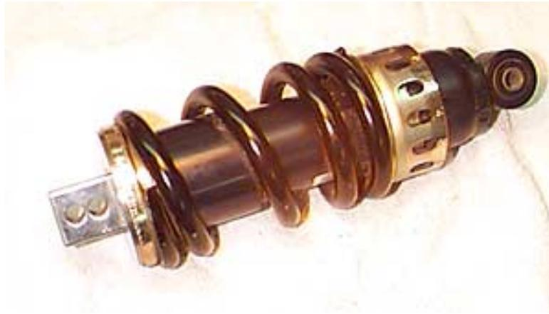
**11.** Reassemble the bike in reverse order. Using the hole farthest towards the end of the shock yields approximately 1.5" of lowering, the hole closer to the shock provides approximately 2.5" of lowering.
