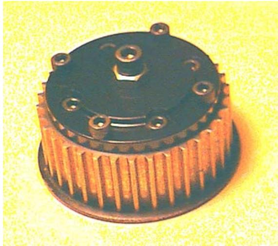
Turn the pulley over in your hand, drop in a deep well socket, and tap with a mallet. The cap will easily pop off, and should require no additional force/prying. See below...
