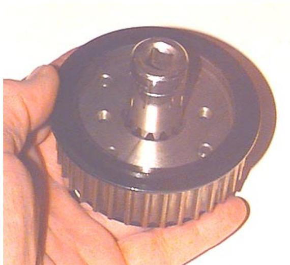
Once the cap is removed, turn the pulley back over and observe the internal features of this component. Using a 5mm allen wrench, remove the two small allen bolts and keeper halves as shown in the photo below. These are the two bolts located adjacent to the splined hole in the center of the pulley assembly, these secure the keeper assembly. See below...
