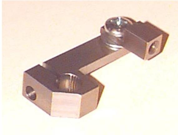
Slip the linkage onto the transmission shifter shaft as in the photo below...with the flat arm facing outward, and being **STRAIGHT DOWN**. This is VERY important. If you have a problem with this, do not attempt to operate the bike until you contact Scootworks Tech Support. It should be installed as in the photo below...
