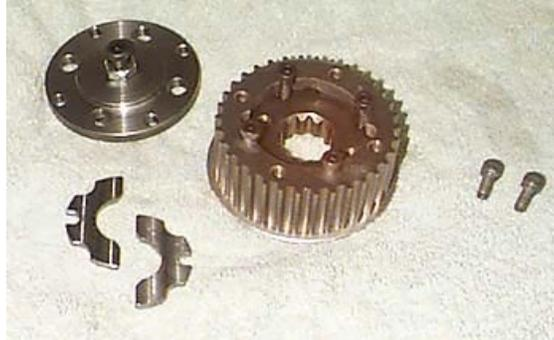
Notice a **small** groove around the inner edge of the pulley assembly, where the center splined core meets the outer toothed portion. Slip the new keeper halves into the groove mentioned above, away from the shaft opening. (DO NOT reuse the splined metal retainer that was originally installed on your factory sprocket). A small amount of grease will help hold these keepers in place until the pulley is installed on the shaft.
