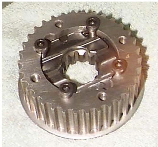
Observe the picture below. The two keeper halves are installed on the pulley, but not secured with the allen head screws. This is how the assembled unit will look when the keepers are in place. See below...
