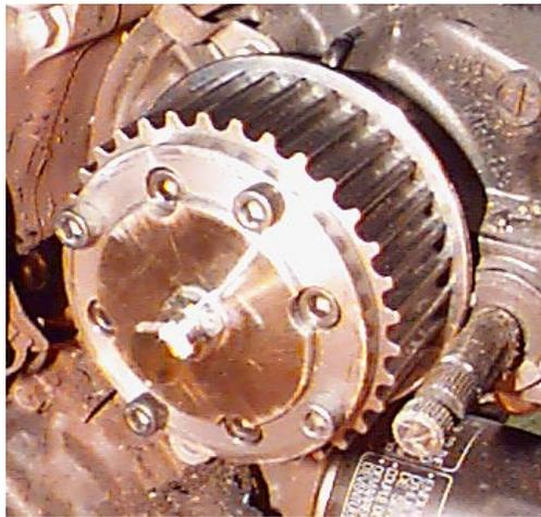
**21.** Pull the belt up and over the front pulley. The photo below shows the correct routing for the belt, in relationship to the splined shifter shaft...
