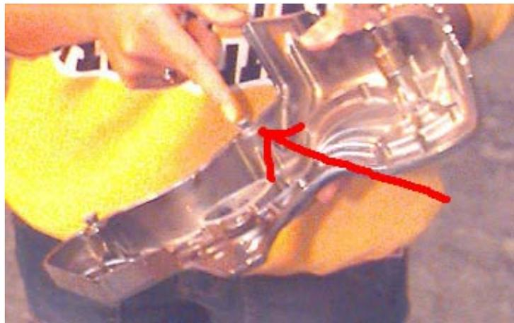
Reinstall the cover on the bike, and view from below to make sure the pegs are shortened enough to provide adequate clearance for the belt. The rubber grommets are mounted on small sheet metal tabs attached to the frame, and may need to be moved a small amount if clearance is an issue. The belt doesn't move from side to side, so only a small amount of clearance is required.
