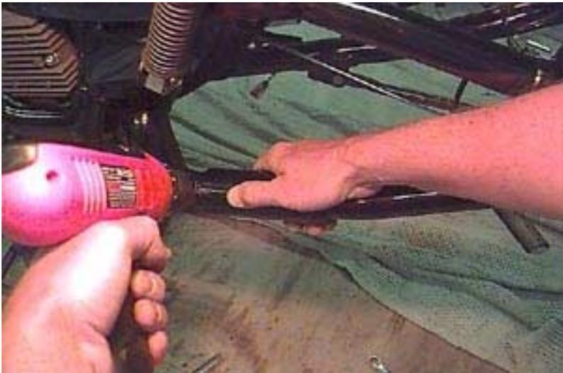
Once completed, you should have a cut and drilled swingarm that resembles the photo below. Place the Gateway sections aside for use a little later in this procedure.
