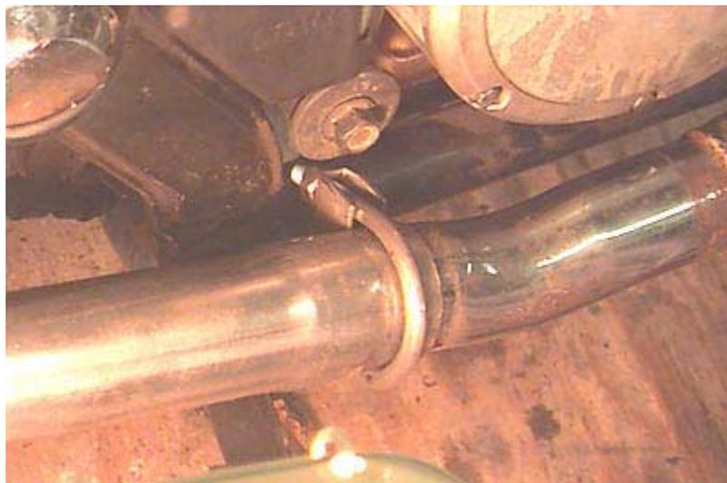
7. Next, wrap a strip of foil tape around the point of connection between the rear of the exhaust bypass tube and the front of the chrome muffler chamber. Slip one of the 3 remaining muffler clamps into position as shown in the photo below. Using a ½” wrench, alternately tighten both of the nuts on the clamp until no loose motion is detected in the junction between the muffler and exhaust bypass tube. This will require some compression of the tubing by the clamp.
