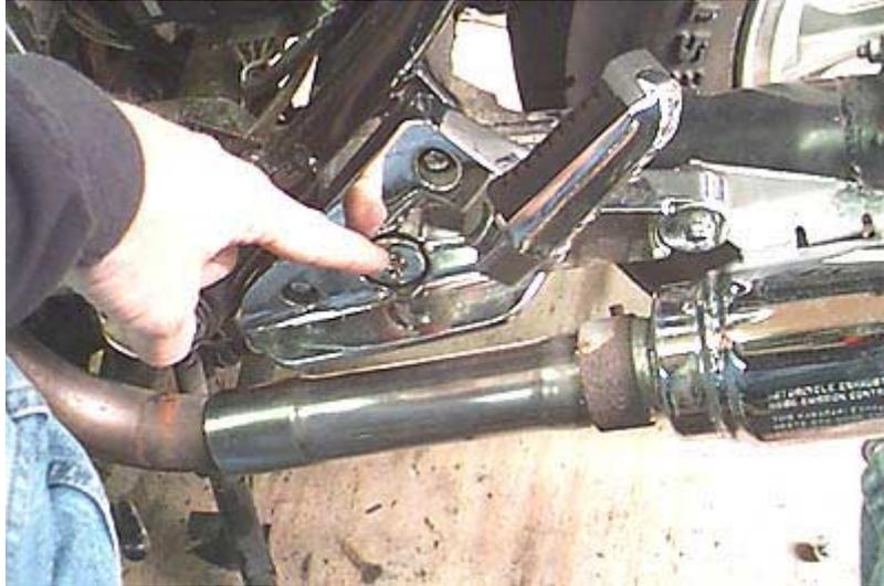
4. Inspect the two supplied aluminized exhaust bypass tubes. One tube is straight, while one tube has a bend at one end. The tube with a bend, is for installation on the RH side of the motorcycle. Slip this pipe onto the RH engine exhaust header, with the bend towards the rear of the motorcycle. Rotate the pipe so the bend is nearly parallel to the ground, as observed in the following photo. Do not install clamps or tighten at this time.
