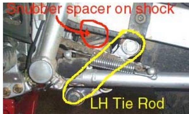
Below is another picture, better exposing the orange rubber snubber on the lower shock absorber rod... This is where the snubber spacers are installed, but don't do it just yet...there's more info on this later in the instructions.
