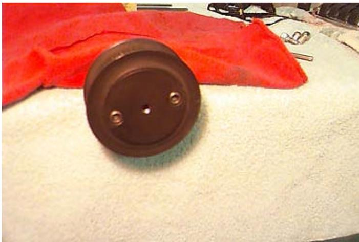
8. Removal of pulley assembly: The keeper retainer cap has a 1/4-20 hole tapped into its center. Remove the two 1/4-20 bolts securing the cap, and thread one into the center opening. Turning it in, against the end of the shaft, will easily push the cap off of the pulley assembly, exposing the keepers and engine output shaft.
