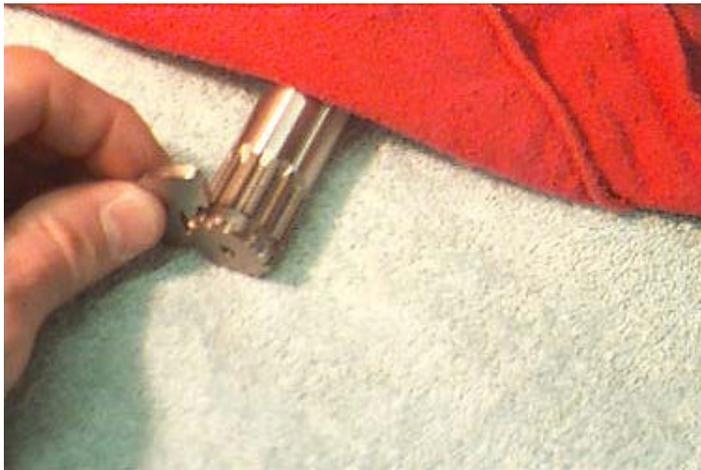
4. Lightly lubricate the splines on the engine output shaft, and the mating splines in the drive pulley assembly. Slide the drive pulley onto the engine output shaft, until the entire retainer groove is exposed on the front side of the pulley. The edge of the retainer groove closest to the engine should be approximately flush with the outward face of the drive pulley's splined inner hub. Notice the photo below for proper alignment.
