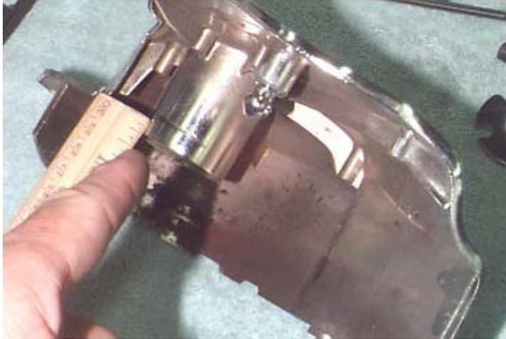
3. For best explanation and photography, an engine output shaft was used to describe the assembly of the front drive pulley assembly. The engine output shaft is the shaft that originally supported the OEM drive sprocket. In the photo below, notice the retainer groove in the engine output shaft. This is the groove where the new keepers will be installed in the following steps.
