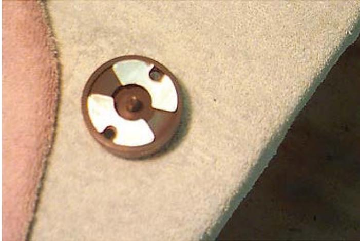
7. Once the keepers are in place, install the cap into the pulley assembly. Make sure the cap is pulled down squarely into the pulley assembly with the 1/4-20 allen bolts supplied. Apply a small amount of medium strength thread lock to the 1/4-20 allen bolts, and install with a 3/16" allen wrench until tight. Observe the photo below for correct final cap installation.
