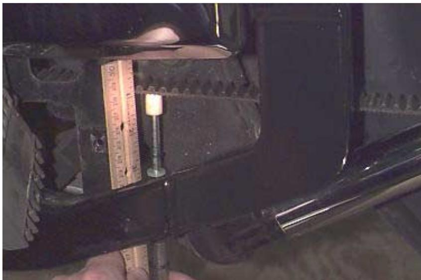
7. Once adjusted, we recommend that you perform is what we call a "pick check". When the belt is "picked" along the edge like a guitar string, it will generate a tone. Observe this when the belt drive installation is new, and use it as a point of reference during the life of your belt. It may sound silly, but it has held true on all of the systems I've installed locally over the last few years, and is a common practice among those who service belt driven motorcycles.
