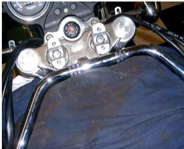
6 While holding the factory risers. Remove the riser bolt nuts. Remove the factory risers. The bolts are tight fit to the rubber dampeners. You may have to use a wooden dowel or other device to drive the bolts up and out of the triple tree. Do not use anything metal, this will damage the threads of the bolts. Just in case you ever wanted to put the riser back on stock height.
