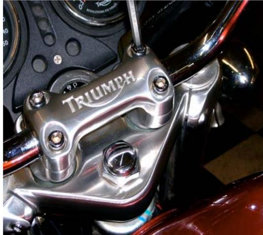
5 When the bridge is removed swing the bars down and rest them on the fuel tank cover.
