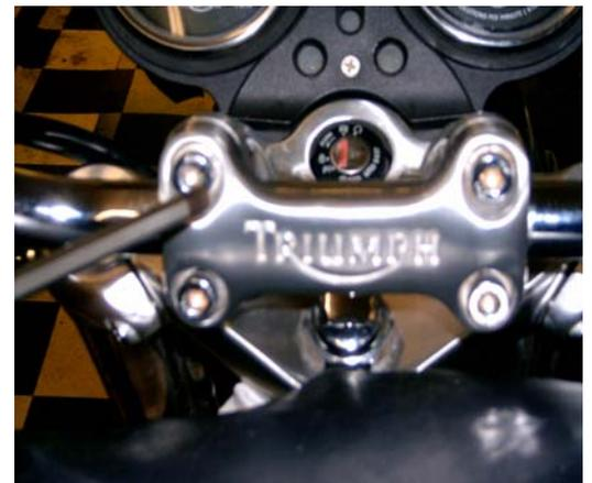
9 With the bridge tightened down, twist the bars left or right to align the bar with the triple tree. When you have the bar aligned with the tree, tighten the bottom riser bolts below the triple tree to 20 ft/lbs. **DO NOT USE ANY THREAD LOCKING COMPOUND ON THE STUDS OR NUTS.**
