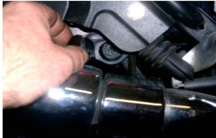
3. Loosen the three bolts using a T55 torx socket bit and a 19mm wrench. Remove the bottom bolt, and the nuts from the upper bolts.
