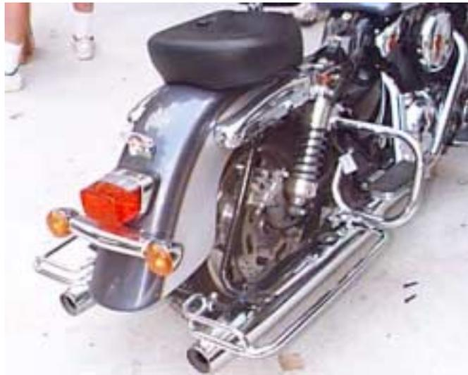
**3.** Slip the Tour Pack mount into position, over the fender rails. Insure the internal structure that runs across the underside of the mount slips down **AHEAD** of the chrome license plate mount (towards the front of the bike), as seen in the picture below.
