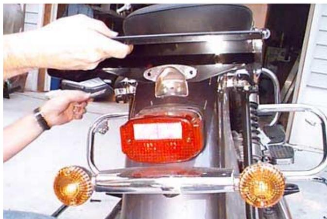
4. Reinstall the 6 (3 each side) bolts through the sides of the Tour Pack mount and into the fender rails. This is sometimes a bit challenging, as the Tour Pack mount is jig welded for accuracy, and often the fender rails on many motorcycles aren't in perfect alignment. Twist the mount slightly (if needed) to allow the each of the bolts to be threaded partially into their respective sockets. Do not tighten at this time!
