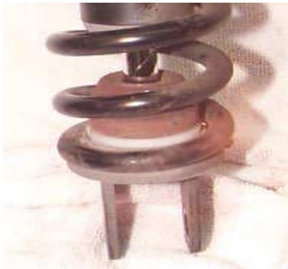
**13.** Reinstall the shock absorber in its upper mounting bracket. Torque this bolt to specification (**43ft/lbs**) at this time.
