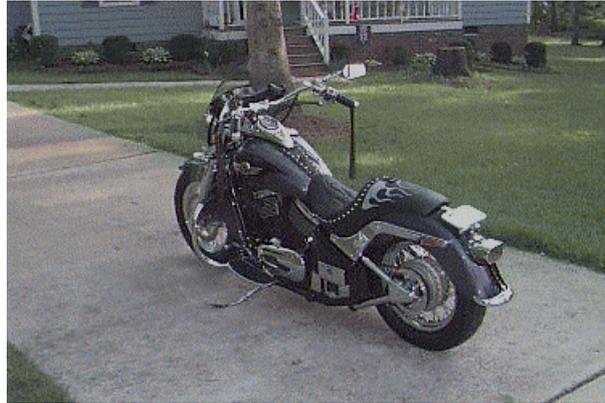
A simple method to alter the angle of the stand with a torch is to heat the kickstand, just below the lower spring tab, until the kickstand is soft enough to bend. Heat the kickstand until red hot in the desired location of bend. Lean the bike against the stand until the desired angle is obtained, then allow the stand to cool on its own. I've altered many kickstands with this method successfully, and never had a failure.
