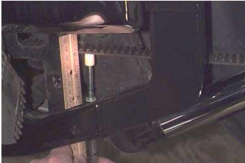
Once adjusted, retighten the axle to 72 ft/lbs. and reinstall the cotter pin, retighten the drum locking bar to 25 ft/lbs. and reinstall the cotter pin, reinstall the voltage regulator, and lock the 12mm and 14mm rear wheel adjuster nuts together.
