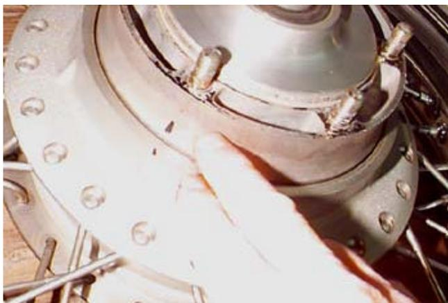
Test fit the new rear pulley on the hub of the wheel. Install the deep side of the pulley towards the wheel.
